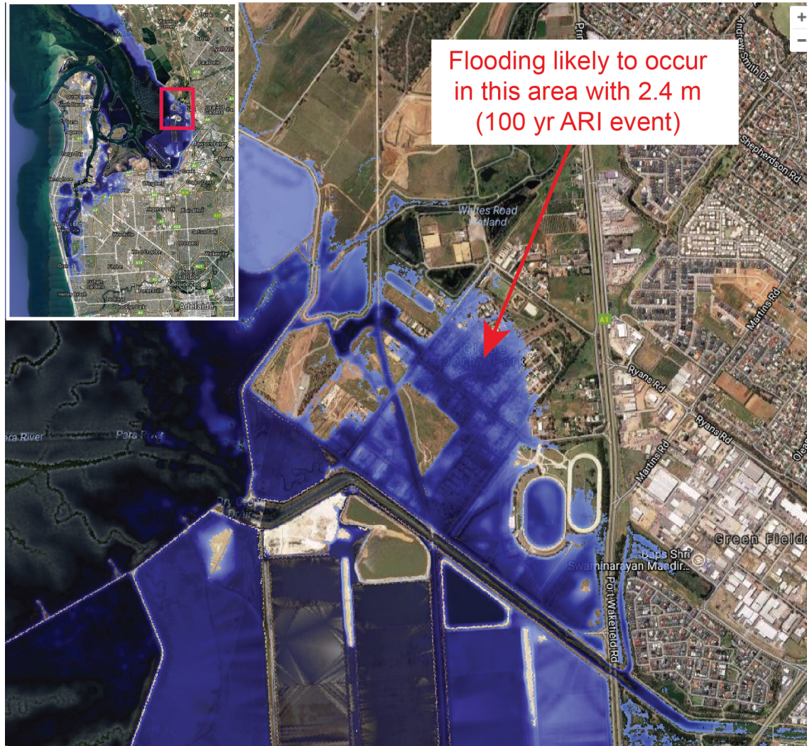
FIGURE 13. ZOOM VIEW OF POTENTIAL INUNDATION IN GREEN FIELDS AREA OF ADELAIDE FOR 100 YR ARI (2.4 M) EVENT, SHOWING LOW-LYING AREAS WHERE INUNDATION IS LIKELY FOR THIS WATER LEVEL.
